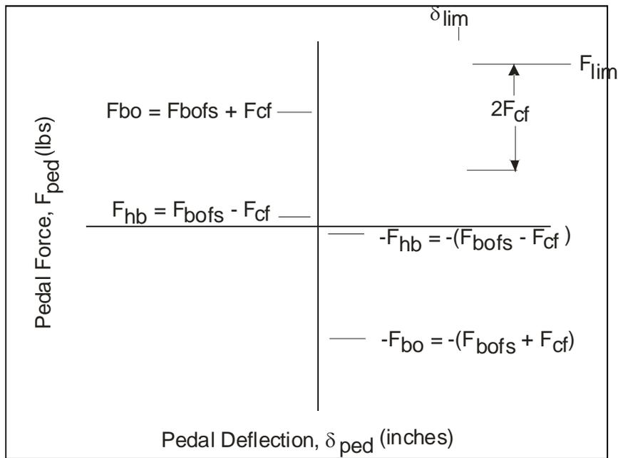
**Figure 3 Definitions for Rudder Feel System Parameters**
