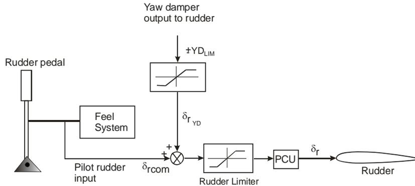
Note: Yaw damper input to rudder is restricted by magnitude of pilot input
