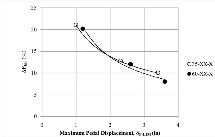
**Figure 7 Excess Vertical Stabilizer Force vs. Pedal-Throw**
