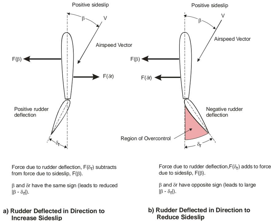
**Figure 1 Vertical Stabilizer Loads and Overcontrol Region**
