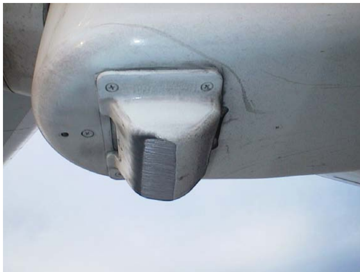
Figure 14 Tailskid Following Tailstrike
