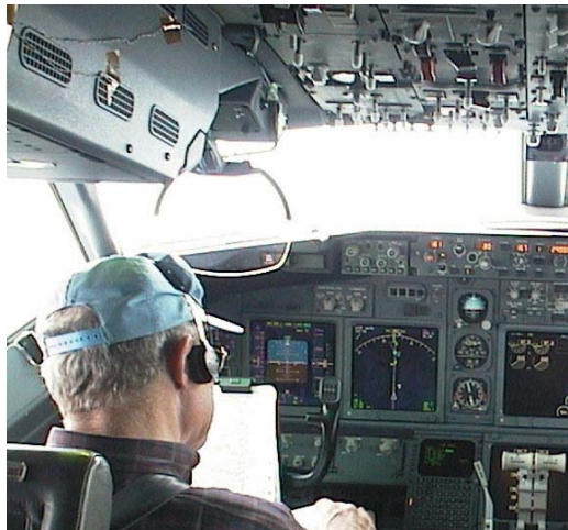
Figure 4 VGS Installation in Boeing 737-800
