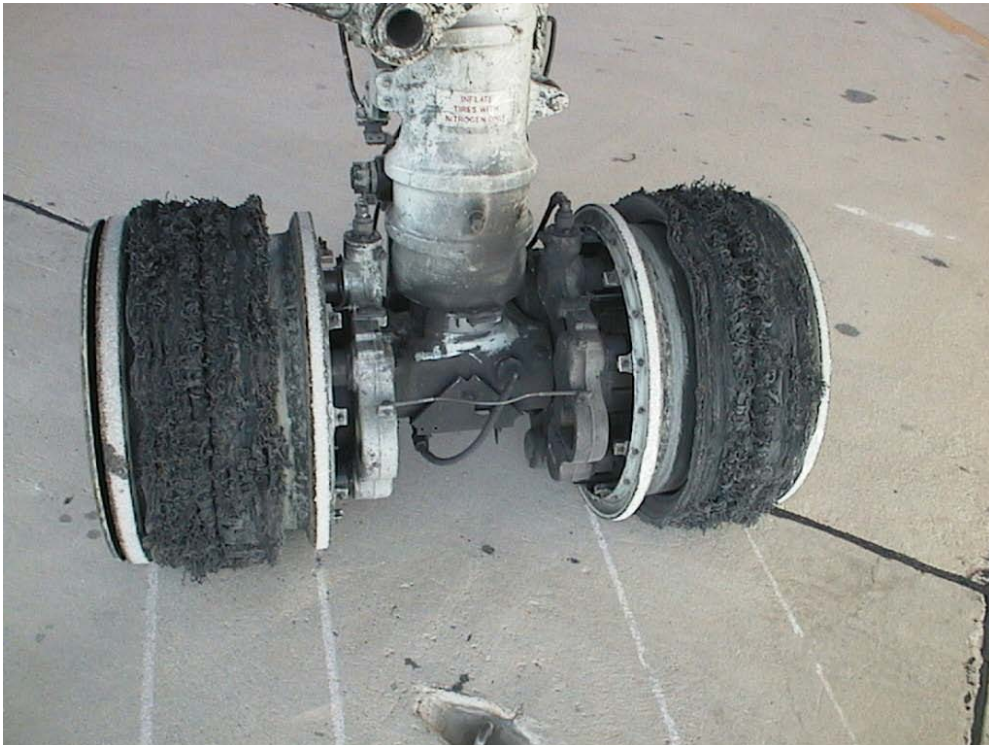
Figure 5 Blown Tires – Too many landings and not enough cooling
