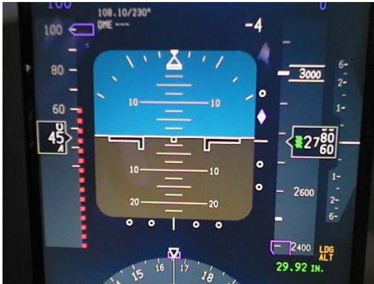
Figure 6 Head Down Primary Flight Display – Boeing 737-800
