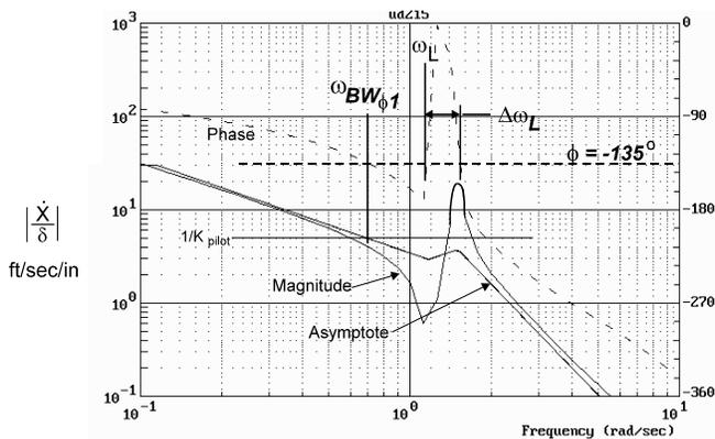
Figure 4 Definition of  $\omega_{BW_{\phi_1}}$  and  $\Delta\omega_L$
